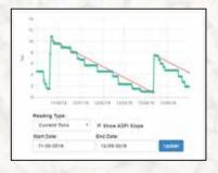
A chart showing sensor level readings converted to tons overlays the ADFI slope indicating consumption and filling, generated for a specific date range. Charts can be created based on other reading types including delivery capacity, distance, percent full, ring space, and sensor battery life. Drilling down further, the most recent sensor reading is timestamped, with reporting on all bin parameters.
